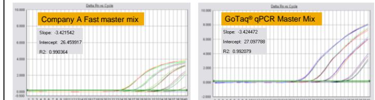
GAPDH amplified from 0.01 – 10 ng human gDNA with GoTaq® qPCR Master Mix and Company A Fast master mix, using the ABI 7500 FAST default cycling parameters: Activation: 95°C for 20 sec. 40 cycles: Denaturation: 95°C for 3 sec Anneal/Extend: 60°C for 30 sec. Data shows GoTaq® qPCR Master Mix is compatible with FAST cycling parameters as is.
