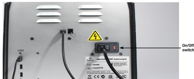
**Figure 13. The On/Off switch.**
