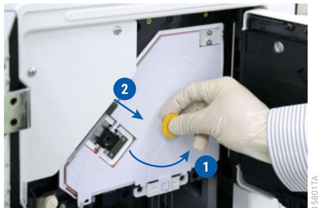
Figure 41. Removing the capillary cartridge.
