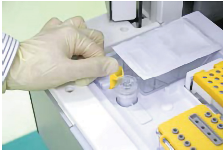
Figure 29. Removing old polymer cartridge.
